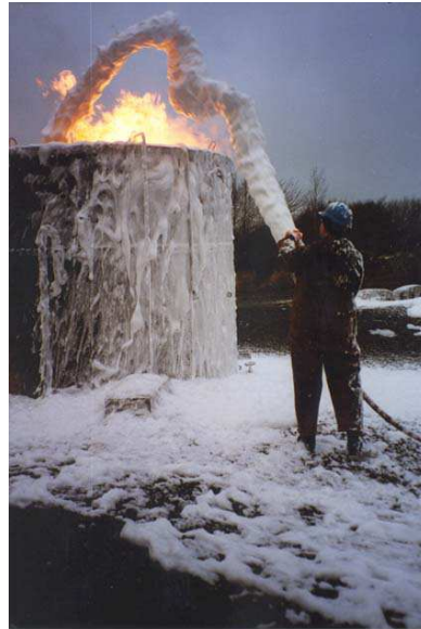
Figure 2: A fire extinguishing foam used on a burning hydrocarbon tank. Foams are particularly useful in that case since they cover the liquid fuel, rather than sinking into it, as water would do. Photo: Mattias Georgsson.
