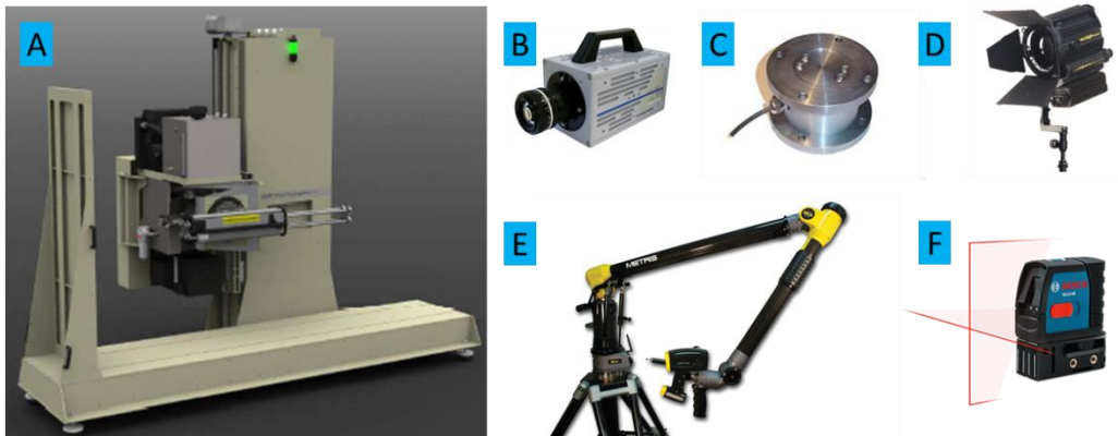
Figure 2-6 : Main instrumentation on the ex-vivo protocol. A. Impact Machine (LF Technologies France), B. High-speed recording camera (FASTCAM SA3, Photron, Japan). C. Six-axis sensor (105515TF, Humanetics, Germany). D. projector (400D, Dedolight, Germany). E. Laser arm scan (Nikon, Japon). F. Positioning laser.
