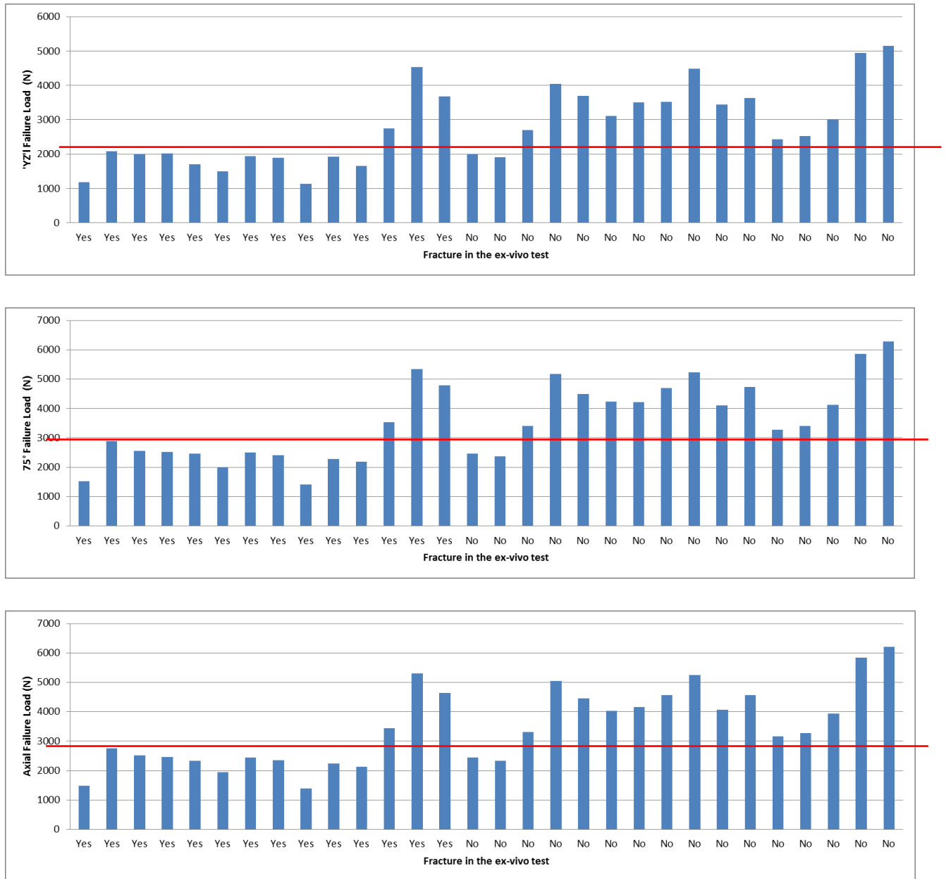
Figure 3-15 : Evaluation of the ratio Failure Load over the fractured and non-fractured cases at the first impact of the ex-vivo experiment Chapter 2. This figure presents the results for 1) Top: the model 'YZ' (-45°), 2) Middle: the fall case model (75°) and 3) Bottom: the axial model (standart HR-pQCT).
