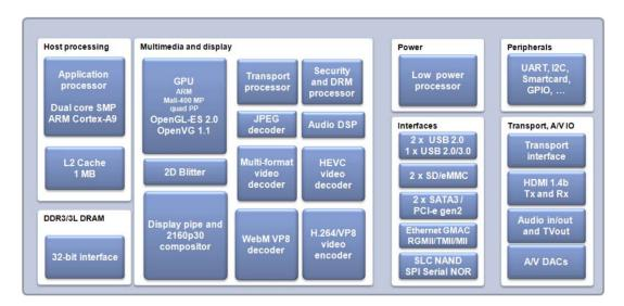
FIGURE 2.2: Block diagram of STMicroelectronics' STiH412 MPSoC for set-top boxes.
