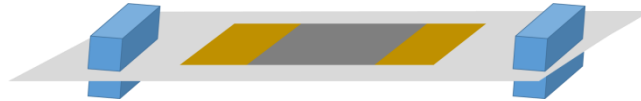
Figure IV.2.4 Preparation of the strain gauge to ensure the transmission of the deformation from the concrete matrix to the embedded sensor.
