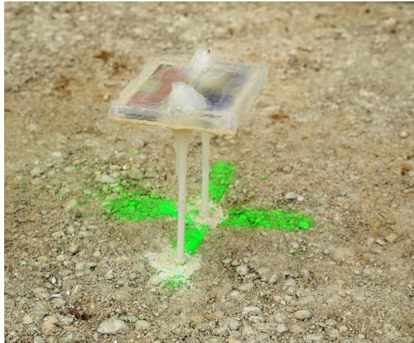
Figure IV.2.6 Embedded wireless platform
