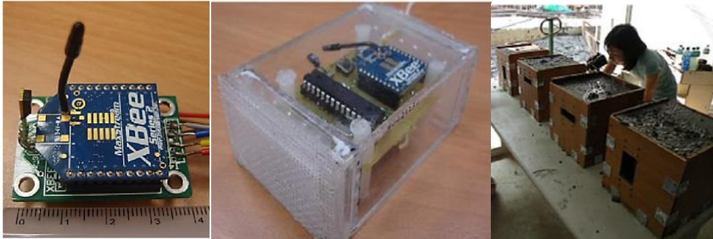
Figure I.1.4 Radio Frequency Integrated Circuit (RFIC) sensor to measure temperature and humidity inside concrete structures (Chang & Hung, 2012)
