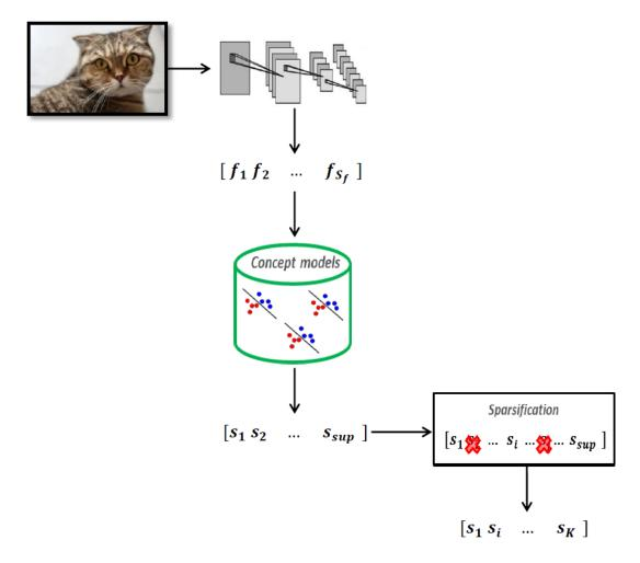
FIGURE 4.1: Illustration of the Semfeat extraction process.
