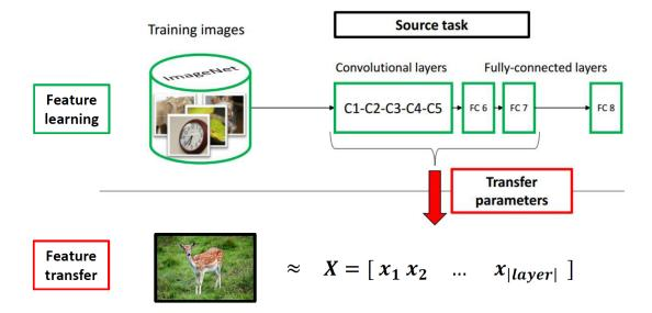
FIGURE 3.1: Transferring parameters of a CNN. Adaptation of the framework depicted in [31]. First, the network is trained on the source task (ImageNet classification, top row) with a large amount of available labeled images. Pre-trained parameters of the internal layers of the network are then used as descriptors for images in different tasks.
