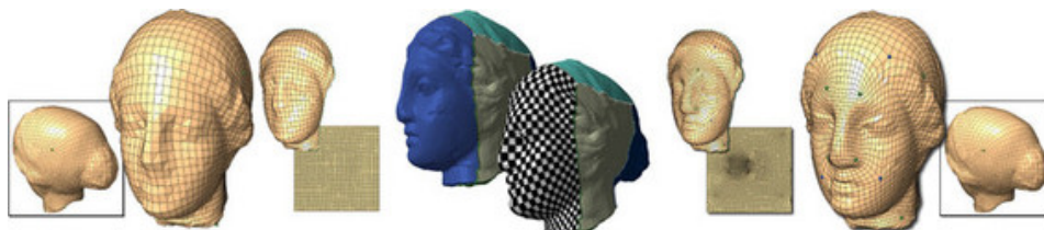
Figure 7.6 – A coarse quadrangulation is extracted from an existing quad-mesh and parameterized (middle). The face is locally improved by connectivity texturing to better capture the nose (right) with no impact on the rest of the mesh (insets).
