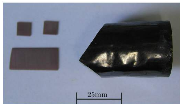
Figure 2.10: 0.71PMN-0.29PT crystal grown [Luo et al., 2009].
