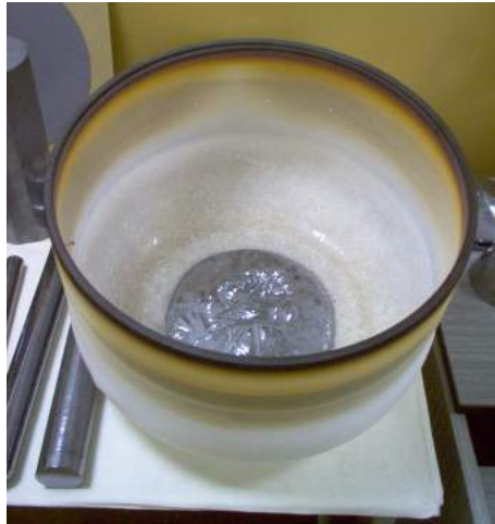
Figure 2.4: A ceramic crucible used in crystal growth.
