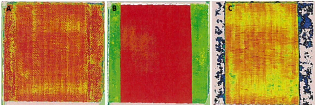
Figure 150: non-destructive testing of a composite plate. A) single transmission attenuation (dB) ; B) single transmission time of flight (mm) ; C) double transmission attenuation (dB).
