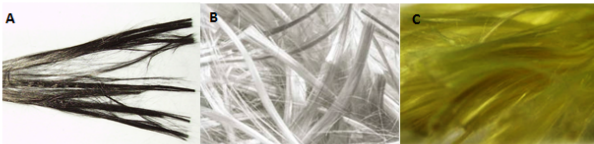
Figure 2: different types of fibres used as reinforcement for polymer matrix composites. A) carbon ; B) E-glass ; C) aramid.
