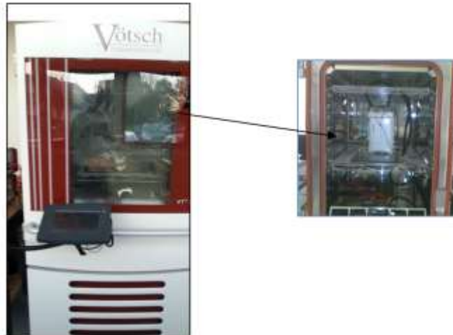
Figure 3.15: The pouch cell battery in the climatic chamber
