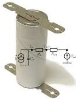
Figure 2.8: Simplified thermal ECM for small cell [74]
