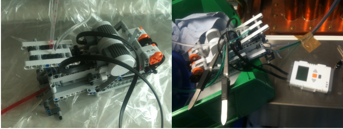
Figure 5.3: Lego unit modeling the contrast pump. Left: Oscillatory tube compressor allowing the modulation of the volumetric flow ratio between contrast and saline solution. Right: Lego unit on top of the MPI Faraday cage, during the flow experiment.
