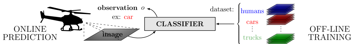
Figure 3 – Example of an observation method in a robotic context: the robot, here a drone, is equipped with a camera and uses a classifier computed from a image dataset (as NORB, see Figure 4): such a classifier is described in Figure 5. The classifier is generated before the mission (off-line) with a image dataset (see the right part of the illustration), and the classifier output is used during the mission (online) as an observation, for the agent (see the left part). Here, observations are thus generated by computer vision means.
