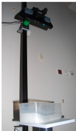
FIGURE 3.9 – Experimental setup with the Kinect depth sensor
