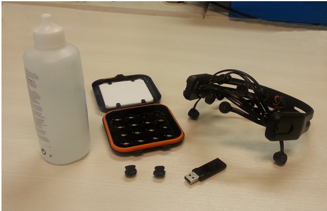
Figure 2.4.5: From right to left: the device adopted (Emotiv EEG) with its USB receiver, electrodes and saline solution.
