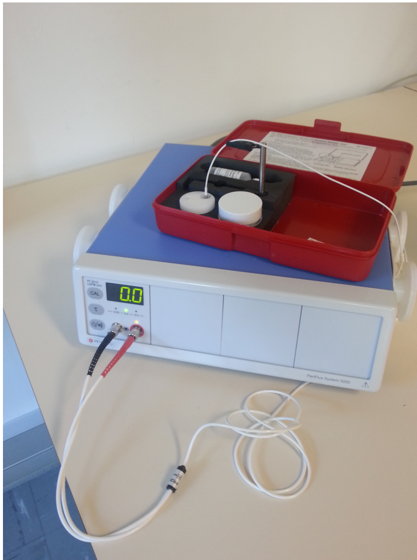
Figure 2.4.2: The PERIMED LDPM device in our laboratory, with it's calibration device on top.
