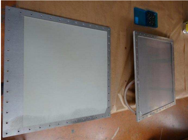
Figure 23 : Resin plate after polymerisation and curing.
