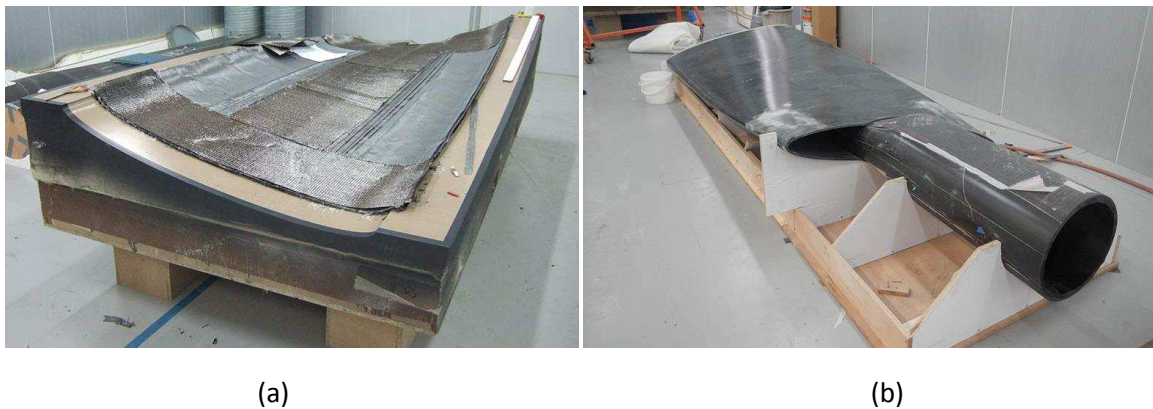
Figure 13: Sabella tidal turbine blade during manufacturing, (a) one side of the blade body before vacuum infusion process and (b) final assembly of spar box and blade bodies [86].
