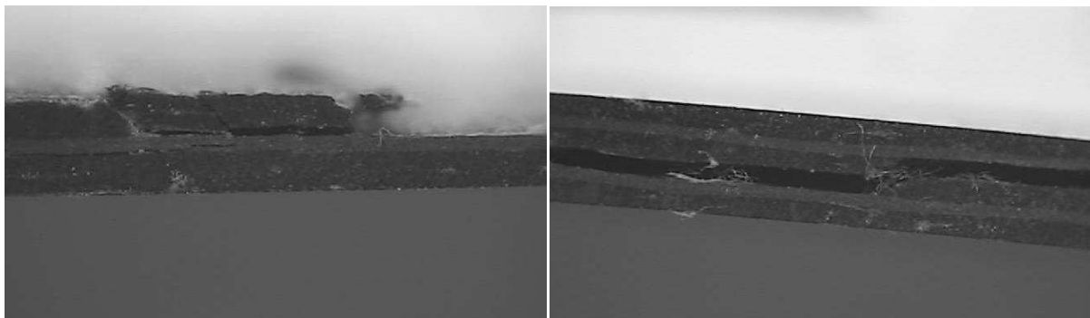
Appendix 32: Examples of fatigue failure mode after sea water ageing on RTM QI 2.8 mm material.
