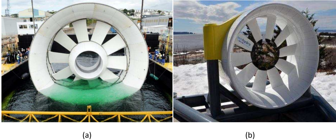
Figure 3: Example of open centre tidal turbine blade developed by OpenHydro and DCNS for the EDF project (a) [14] and the Bay of Fundy (b) [15].
