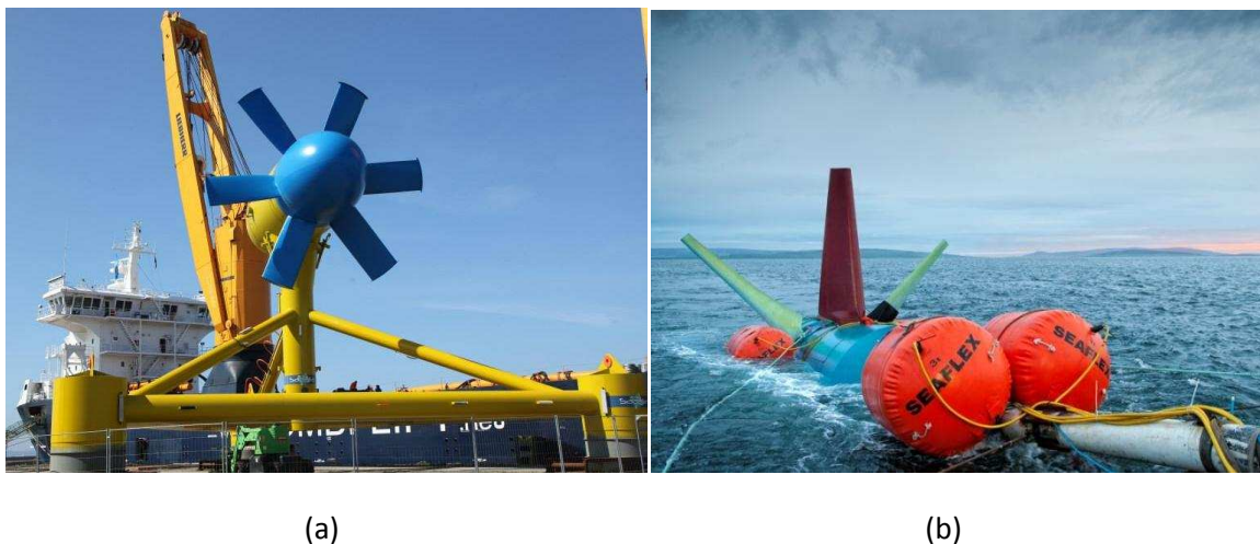
Figure 2: Sabella D10 Tidal turbine (a) and CoRMAT tidal turbine with 4 m RTM blades, courtesy of Airborne Marine and Nautricity Ltd (b).
