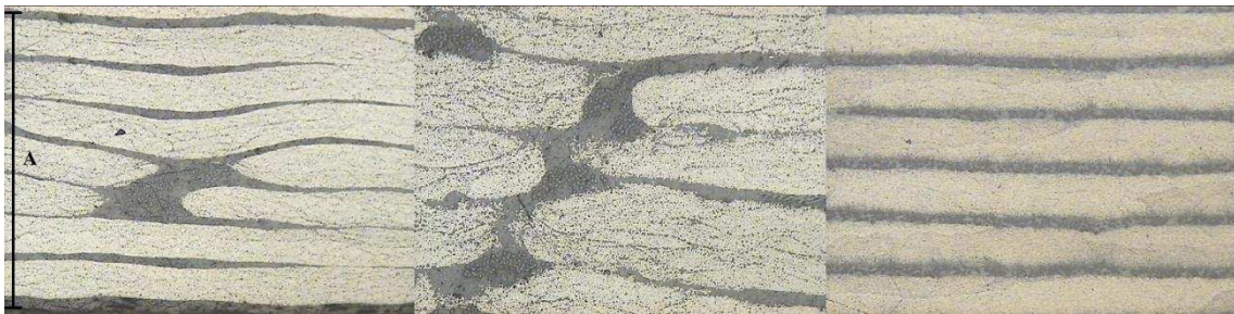
Figure 55: Optical microscope observation of UD samples, left to right, Infused, RTM and Pre-preg materials (dimension A is approximately 1.5 mm, for all three materials).
