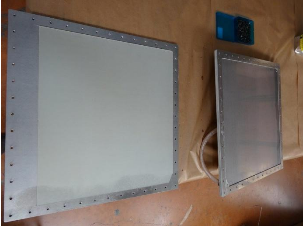
Figure 23 : Resin plate after polymerisation and curing.
