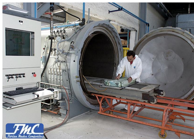
Figure 19 : A pre-preg part under vacuum going into the FMC autoclave, [91].
