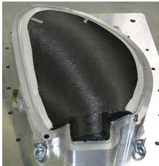
Figure 20 : AMBV (Alkmaar class Mine-hunting vessel) composite propeller and mould engineered by Airborne Marine.
