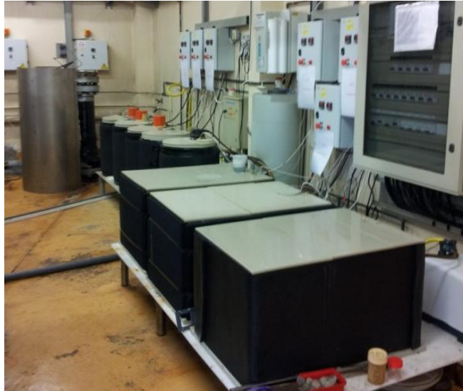
Figure 83: Ifremer sea water ageing tanks with natural and renewed sea water from the bay of Brest.
