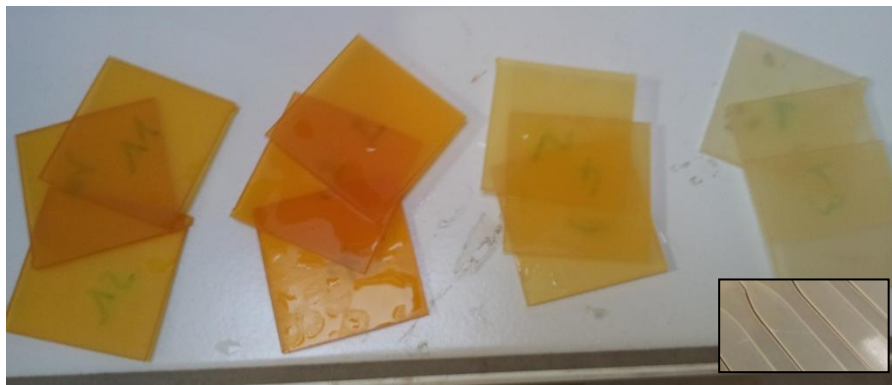
Figure 88: Epoxy resin samples used for weight measurement at 80, 60, 40 and 25°C (left to right) suggesting oxidation of the resin.
