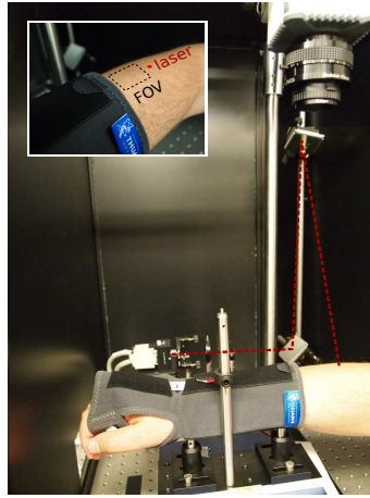
Figure 4.19: The photograph of the setup for the in vivo experiment. The inset figure depicts the approximate location of the source and the field-of-view. Figure reproduced from [110].
