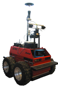
Figure 4.7: LAAS-CNRS Dala robot with an ATRV base
