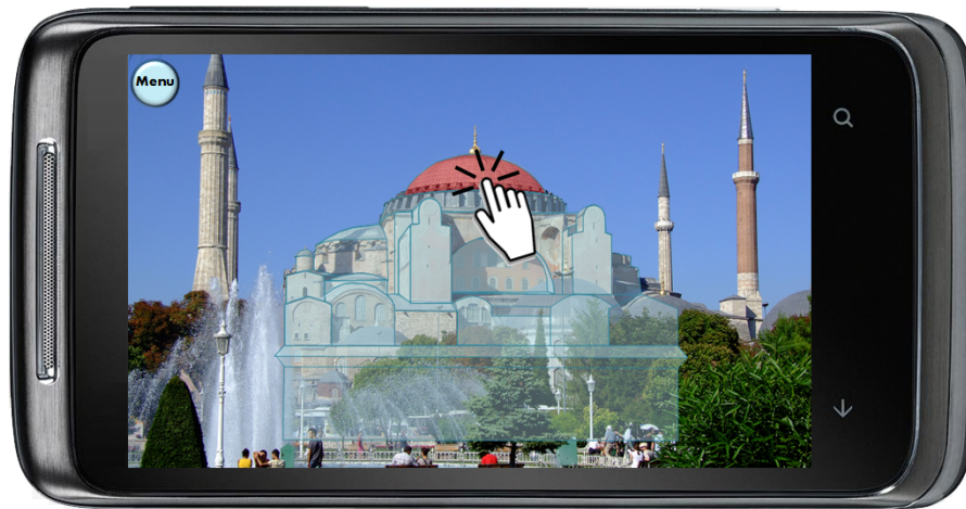
Figure 5.12 – A representation: the parts of the 3D object are rendered in different colors to tell the user that there is some additional information related to these parts of the real world entity. The user interacts with these parts on the screen to access this information.
