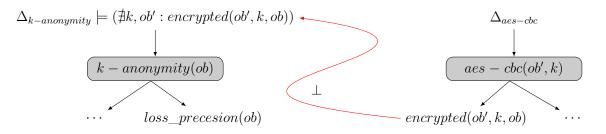
Figure 6.2 – Two conflicting mechanisms: The preconditions of k – anonymity and the effects of aes - cbc are inconsistent.
