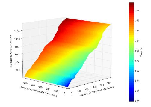
Figure 4.3 – Policy satisfaction evaluation in function of the number of sensitive attributes, the number of threshold constraints, and the number of utility constraints
