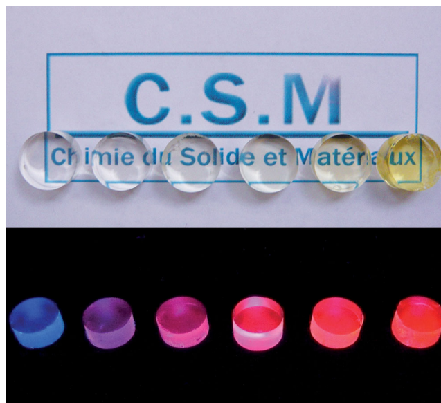
Figure 1. Digital photographs of the \text{Mo}_6 -PMMA hybrid copolymer pellets under visible (top) and UV light (bottom); \lambda_{\text{exc}} = 365 \text{ nm} ; cluster concentrations range from 0 to 0.36 wt% from left to right.
