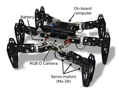
Figure A.1: The hexapod robot, which is used to evaluate the performance of the algorithms proposed in this manuscript.
