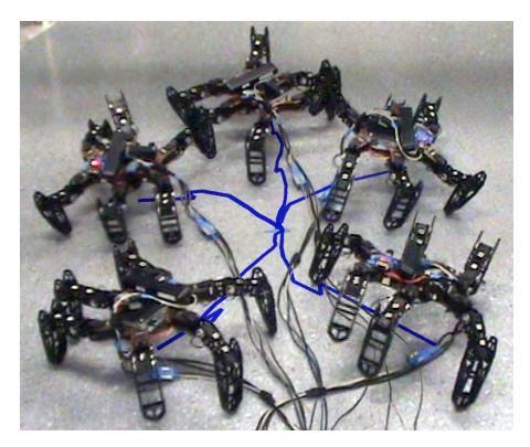
Figure 3.18: Illustration of the results obtained with TBR-Evolution. These 5 typical trajectories correspond to controllers obtained with TBR-Evolution as recorded by the SLAM algorithm. The supplementary video shows a few other examples of controllers.
