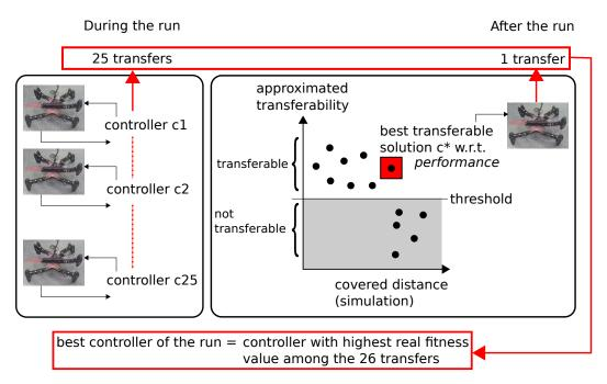
Figure 4.2: Choice of the final solution at the end of the T-Resilience algorithm.
