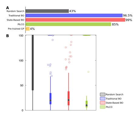
Figure 5.3: Reaching the first target. A) Success rate for reaching the first target with the five compared algorithms. B) Comparison of the number of trials required to reach the first target. The experiment has been replicated 200 times in simulation for each of the tested algorithms.
