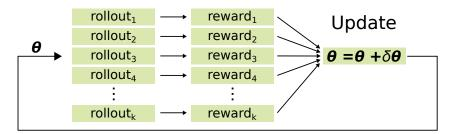
Figure 2.3: Generic Policy Search iteration. The current policy defined with the parameter vector  $\theta$  is used to generate k rollouts thanks to perturbations on the parameters or on the motor commands. Each rollout is evaluated on the system and is associated to a reward value or several intermediate rewards. Based on these rewards, the current policy is updated and the process repeats.
