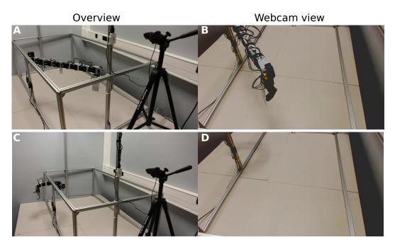
Figure 5.10: Two examples of situation where the laser point is not visible. (A-B) The laser point is too close from the camera and consequently outside the camera's range. (C-D) The laser point is hidden by the pillar of the structure.
