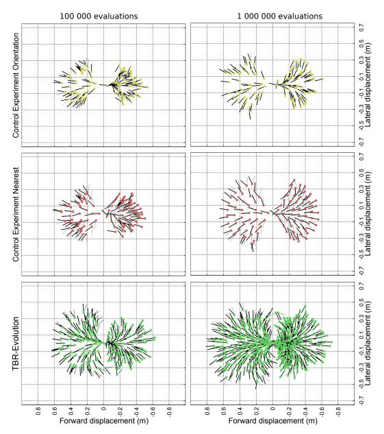
Figure 3.4: Comparison between the typical results of the TBR-Evolution algorithm, the "nearest", and the "orientation" variants. The archives are displayed after 100,000 evaluations (left) and after 1,000,000 evaluations (right). Each dot corresponds to the endpoint of a controller. The solid lines represent the final orientation of the robot for each controller, while the gray dashed lines represent the desired orientation. The orientation errors are the angle between solid and dashed lines.
