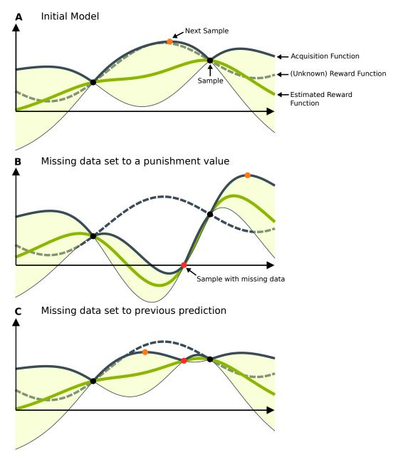
Figure 5.4: Common ways to deals with solutions that cannot be evaluated. (A) Initial model, the performance of the "next sample" cannot be assessed. The two other sub-panels show the impact of commonly used techniques to deal with missing data. (B) Samples with missing data receive a punishment value (here 0), distorting the model as a consequence. (C) Samples with missing data receive the value previously predicted by the model, fixing it to a potentially wrong value.
