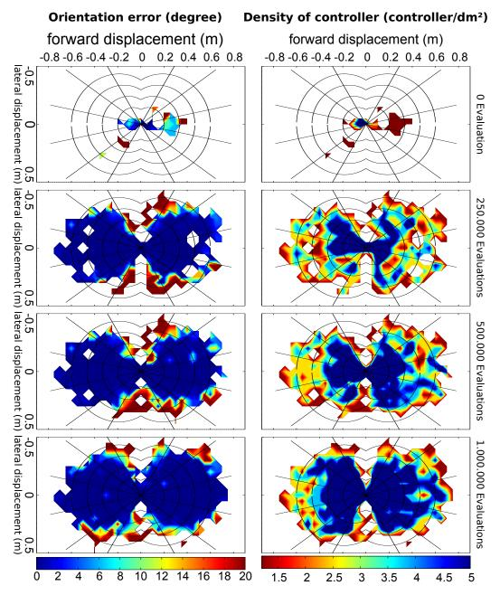
Figure 3.9: (Right) Variation of density of controller (number of controllers per  $dm^2$ ). (Left) Variation of the orientation error (given by the nearest controller) along a typical run in simulation.
