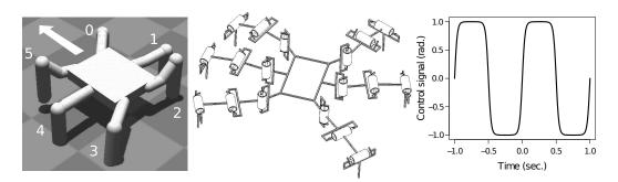
Figure 3.2: (Left) Snapshot of the simulated robot in our ODE-based physics simulator. (Center) Kinematic scheme of the robot. The cylinders represent actuated pivot joints. (Right) Control function  $\gamma(t, \alpha, \phi)$  with  $\alpha = 1$  and  $\phi = 0$ .
