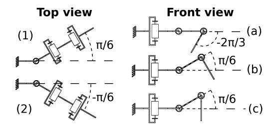
Figure D.1: The six possible actions of a leg that can be tested on the robot: (1,a), (2, a), (1,b), (2, b), (1,c), (2, c).
