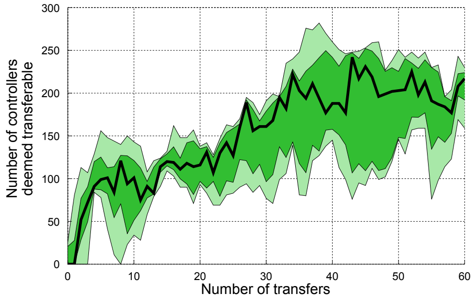
Figure 3.12: Evolution of the number of controllers deemed transferable. At each transfer (i.e. every 50 iterations), the number of controllers with an estimated transferability lower than 15cm is pictured for all the 5 runs. The bold black line represents the median value, the dark region the first and third quartile and the light one the lower and upper bounds. The variability of the curve is due to the periodic transfers, which update the transferability function and thus the estimated transferability values.
