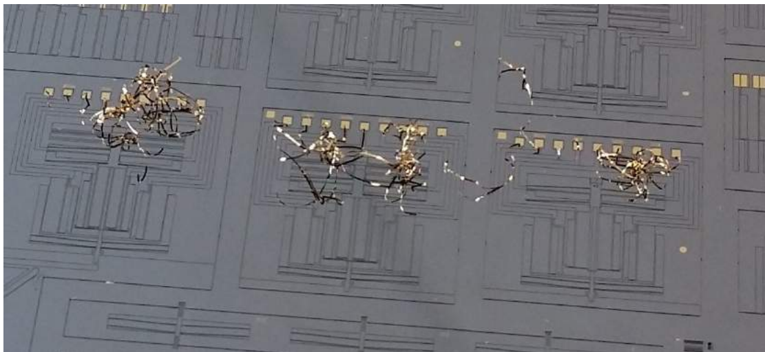
FIGURE 5.17: The gold patterns started to peel off from the wafer after inserting it in the HF solution.
