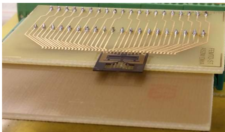
FIGURE 5.32: A multistable module prototype glued and wire bonded on a PCB
