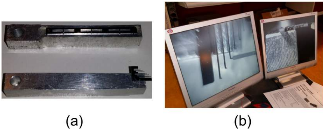
FIGURE 5.23: Curved and rectilinear beam prototypes (a), screens showing a direct image from the side and top of the prototypes and force sensor probe (b).
