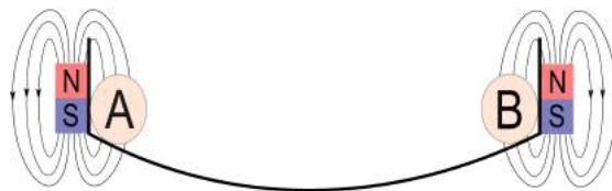
FIGURE 1.10: Holding principle via permanent magnet.
