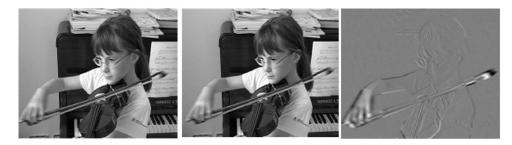
Figure 2-8: (a) Reference picture t (b) Picture to be compressed t+1 (c) difference between pictures
