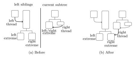
Figure 3.11: Before and after settings threads and updating extreme nodes.
