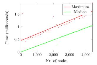
Figure 3.10: Measurements on random trees. The minimum is not shown, as it coincides with the x-axis.
