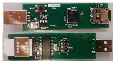
Figure 17: ZED Secure device (front & back)
