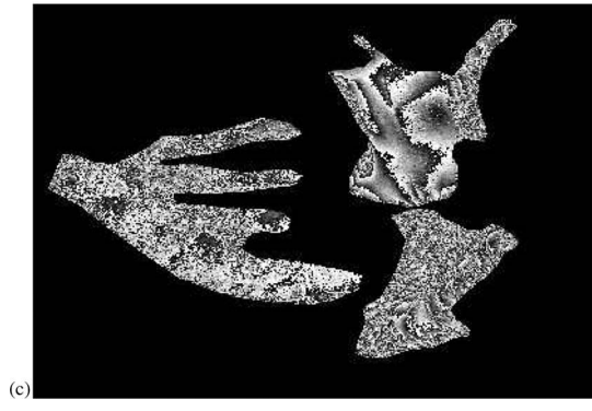
Fig. 2. Wrapped phase difference between interferograms on the Tour, Trient, and Saleina glaciers. (a) \Delta\Phi_{\text{April-March}} . (b) \Delta\Phi_{\text{April-December}} . (c) \Delta\Phi_{\text{April-October}} .
