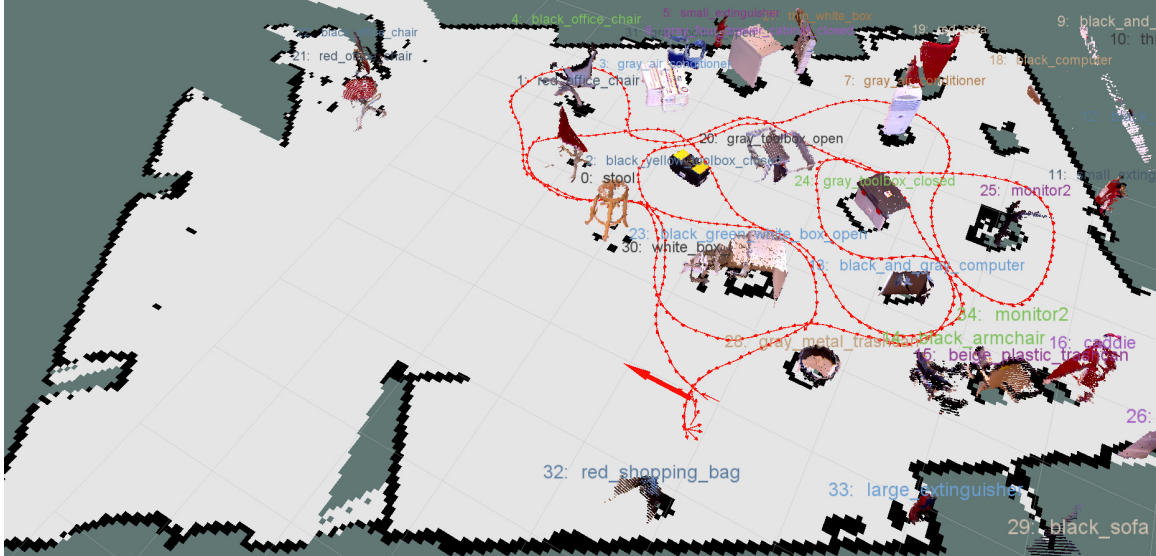
Figure 1-2: A semantic map. The image shows a metric map with semantic annotations. The light region is the mapped regions. It is delimited by a black boundary. The semantic annotations are a snapshot and the name of the objects present in the scene. The object images are hollow because they are the actual point clouds captured by the Kinect. The red trail is the path followed by the robot to produce this map.
