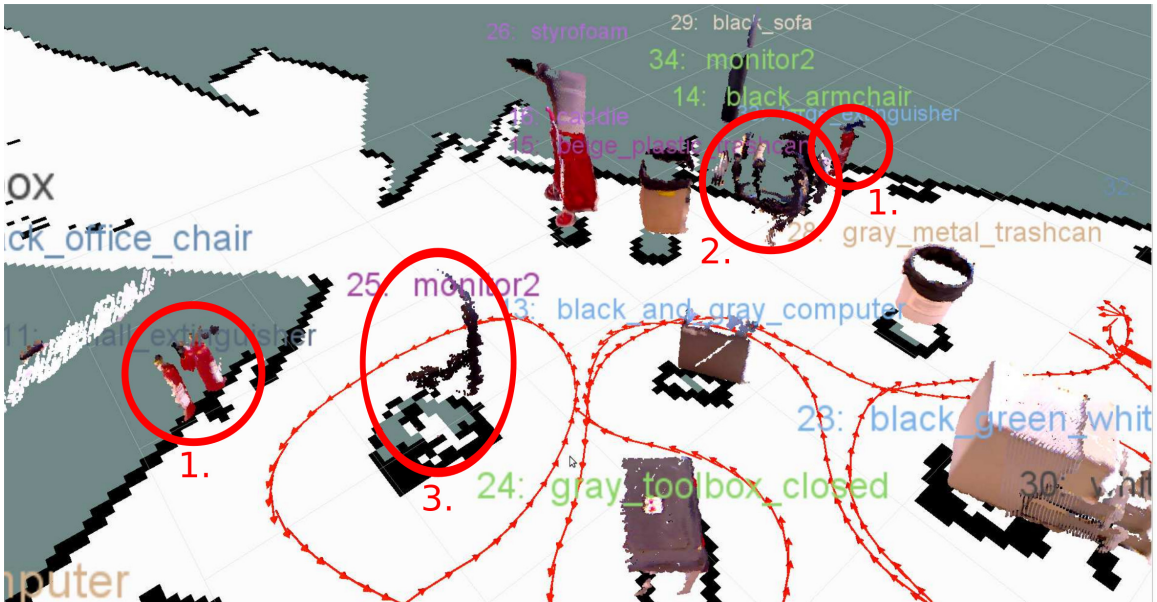
Figure 5-7: Zoom on the semantic map. The numbered red circles indicate interesting points in the map. 1. Successful segmentation of objects in contact with a wall. Also duplication of the extinguisher on the left. 2. Failure to remove background clutter. 3. Incomplete segmentation of a black object.
