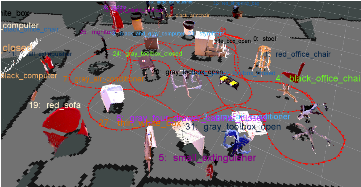
Figure 5-6: The semantic map resulting from the online experiment. The map is built using Hector SLAM and the laser range finder. On top of the maps, all the objects returned by the geometric segmentation algorithm are pictured. The object images are hollow because they are the actual point clouds captured by the Kinect. The red trail is the path followed by the robot. This image is a different view of the semantic map shown in chapter 1, figure 1-2
