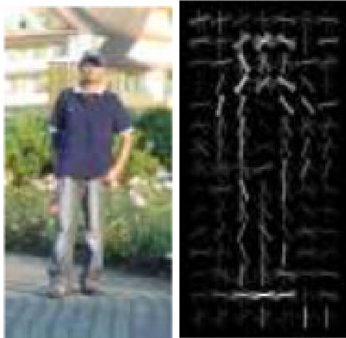
Figure 2-3: HOG feature for pedestrian detection. Left Example of an image of a pedestrian. Right A HOG feature computed over many pedestrian images. The silhouette of a typical pedestrian appears in the feature. The silhouette has two heads due to variations in the pose of the pedestrians in the images used to compute the feature.
