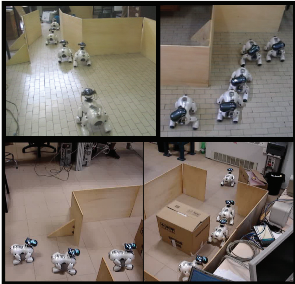
Figure 5.4: Three experiments showing the performance of semi-autonomous navigation. The user drives the robot using a single command: 'go forward' (top left and bottom) and 'go right' (top right).
