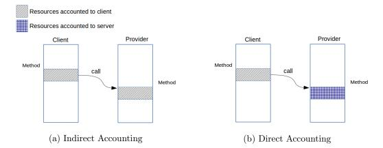
Figure 3.4 – The two mechanisms to account for resource consumption when components interact.
