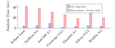
Figure 6.15 – Analysis time for real applications. It shows the time needed to compute an analysis just once. The analysis aims at finding the consumption of the top components
