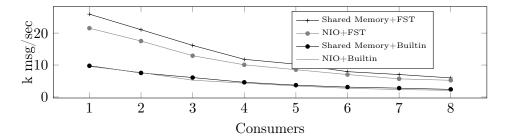
Figure 5.8 – Communication throughput for different channels.
