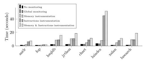
Figure 4.4 – Execution time for tests using the DaCapo Benchmark
