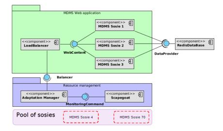
Figure 4.11 – Architecture of MdMS along with Scapegoat and additional components to adapt the system.
