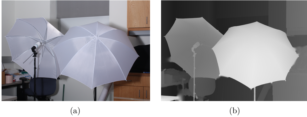
Figure 4.13: (a) Right view and (b) depth map of the considered stereo data set.
