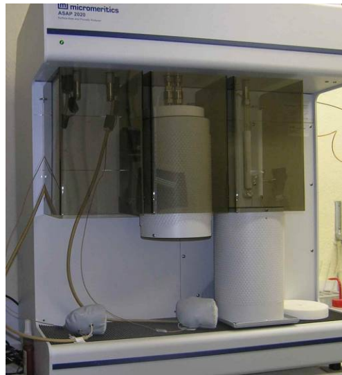
Figure 3.2 Equipment of ASAP 2020 physisorption analyzer
