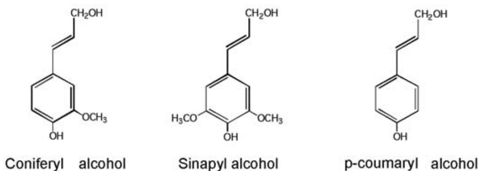
Figure 1.9 Chemical structures of lignin precursors
