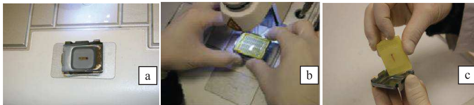
Figure 2.6 (a) Fixing the microcore at the bottom of mold, (b) formation of the paraffin block (c) stripping the paraffin block off (Image: Harroué et al. 2011).
