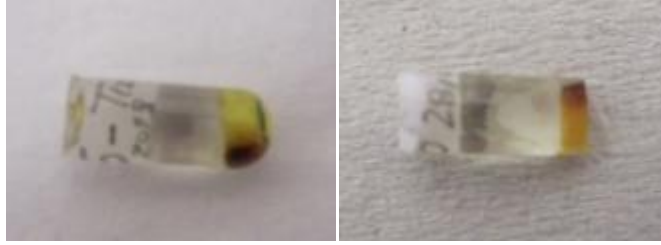
Figure 3.3 (a) resin block before trimming (b) resin block after trimming
