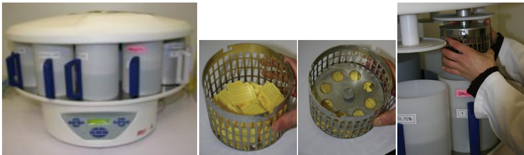
Figure 2.4 Impregnation machine (STP120, Microm)
