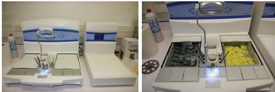
Figure 2.5 Embedding station EC 350-2 (Microm)
