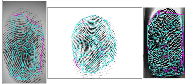
Figure 6.3 – Example of minutiae Delaunay triangulations of 3 different FVC images. NFIQ values are 2, 2 and 1, respectively.
