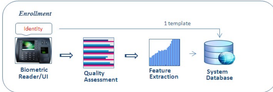
Figure 1.4 – Diagram of enrollment. This is a 4-step operation including reading (capture), quality control, feature extraction and saving.
