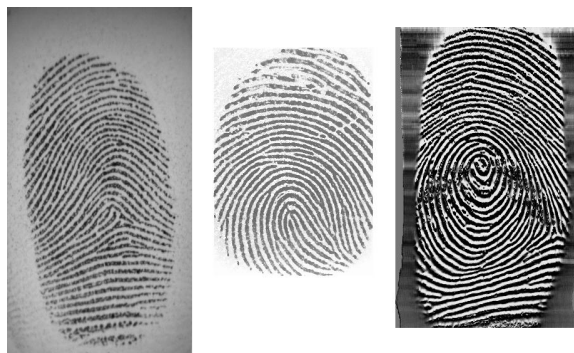
Figure 2.3 – Example of fingerprint images from the FVC databases (from the left to right): optical, capacitive and thermal sweeping. Resolutions are over 500-dpi.
