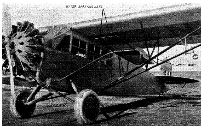
Figure 1.11: Flight Test Apparatus for Vapor Heating Boiler System [138]
