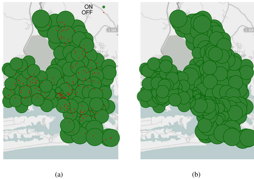
FIGURE 6.2: Configuration of BSs to provide a full geographical coverage over the city with: (a) a switch-on/off scheme, where a BS can be on or off and (b) all-on scheme, where a BS cannot be switched-off. A switched-on BS is represented with a green disk, whose size is an approximation of its actual coverage area, and a switched-off BS is referred to with a red dot.
