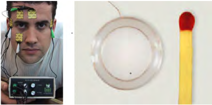
Figure 13: Eye-tracking systems. Left, EOG system from Qubit systems http://www.qubitbiology.com (2010). Right, Magnetic scleral search coil to be placed on the eye.
