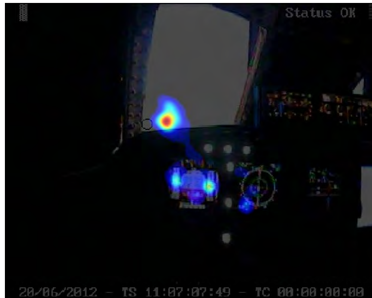
Figure 20: Heat map calculated from eye-tracking data recorded during a period of manual flying in a flight simulator. It highlights the use of the Out Of the Window (OTW) and the speed and altitude indicators on the Primary Flight Display (PFD)
