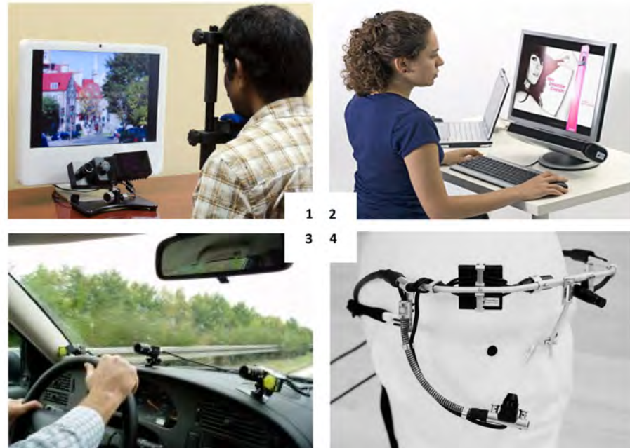
Figure 17: Eye-tracking systems. 1) Fixed and constrained, Eye-link 1000 Plus. The IR projector is the black grid on the right of the system 2) Fixed and remote on a desktop, SMI Red 500, both cameras and IR projectors are embedded under the screen 3) Fixed in a cockpit, Smart Eye Pro, IR flashes are the yellow dots close to the camera 4) Head-mounted, EyeTechSensor, IR flashes are on both sides of the eye camera
