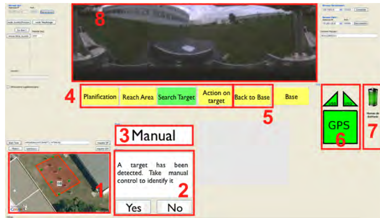
Figure 22: Ground Station Interface: 1) "tactical map", 2) "interactive panel", 3) "mode annunciator", 4) "synoptic", 5) "back to base", 6) "GPS and ultrasound status", 7) "battery status", 8) "panoramic video".
