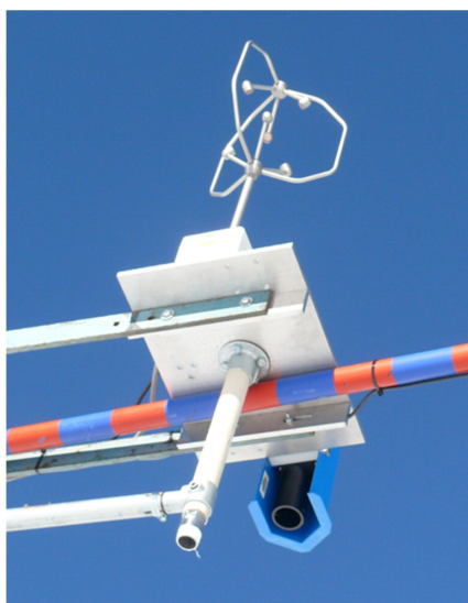
Fig. 4. Ultrasonic anemometer and snow-depth sensor (Jenoptik) (H.Bellot/Irstea).
