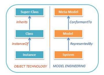
Figure 16. Object technology & Model engineering.
