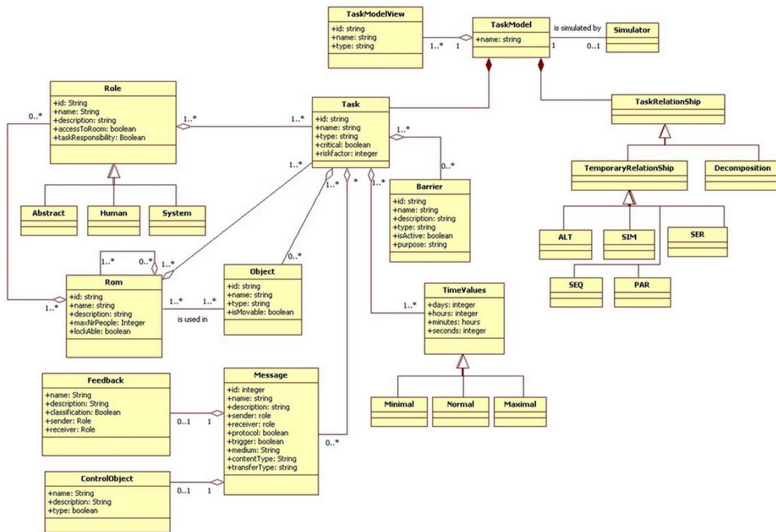
Figure 18. Meta-model of the UsiXML task model.
