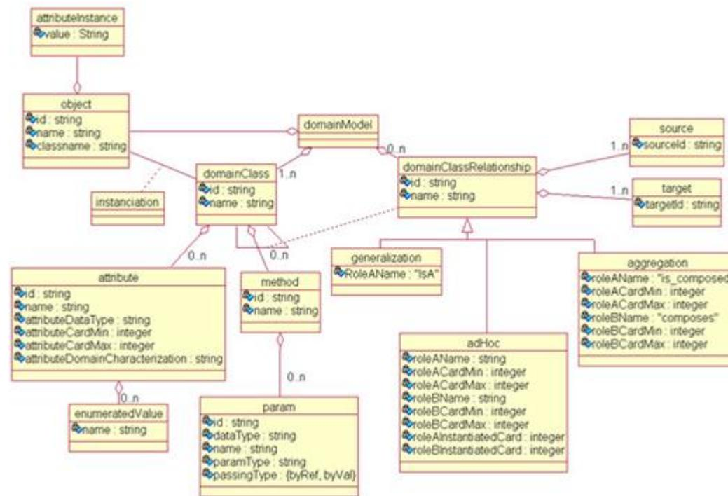
Figure 20. Meta-model of the UsiXML domain model.
