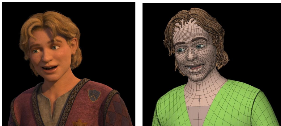
Figure 2.5: Digital objects in computer graphics. Left: The final object is the mesh from the left image with attributes of color and texture added. Image taken from animation film Shrek.
