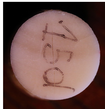
Fig. 5 - Appearance of a vertical crack at the centre of a specimen x_1-F_3 with a 8.12 mm diameter.
