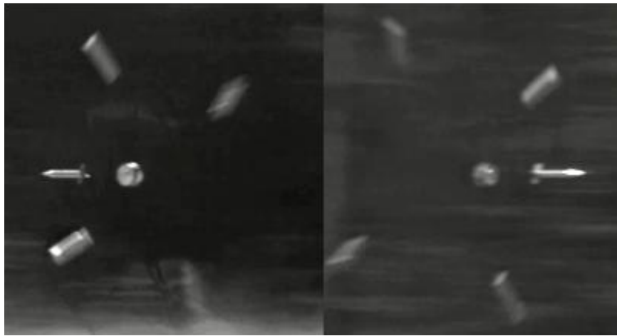
Figure 4.25: Snapshots of sabot separation obtained from the two trajectory trackers
