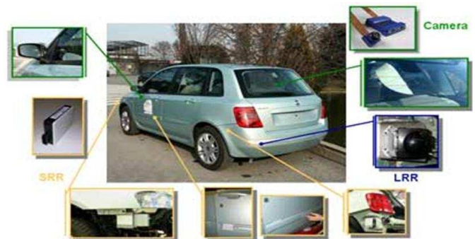
Figure 6 : Set of sensors for vehicle lateral monitoring in Lateralsafe sub-project of PReVENT (three short range radars (SRR, in yellow colour) on each side, one long range radar (LRR, in blue colour), and two cameras (in green colour)).
