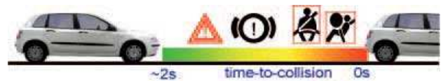
Figure 4 : Pre-crash and collision mitigation as a function of the time-to-collision are illustrated in the figure (APALACI and COMPOSE PReVENT sub-projects).
