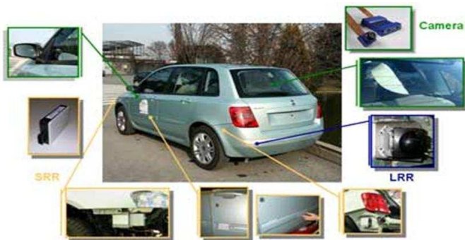
Figure 6 : Set of sensors for vehicle lateral monitoring in Lateralsafe sub-project of PREVENT (three short range radars (SRR, in yellow colour) on each side, one long range radar (LRR, in blue colour), and two cameras (in green colour)).
