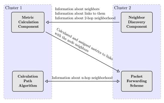
**Figure 4.1:** Semantic schematic of general interactions between different components of a link-state routing protocol for one node.
