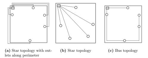
Figure 3.3: Three most conventional in-home wiring topologies
