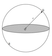
Figure 2.1: Isotropic antenna radiation assuming source model point
