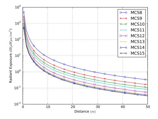
Figure 2.4: Radiant Exposure versus distance from radiating source for different modulation schemes of IEEE 802.11n
