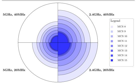
Figure 4.3: Transmission ranges to MCSs mapping
